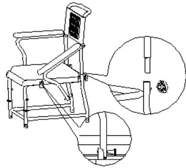
10. The wheels are inserted from below into the frame and can be easily removed again. All wheels are pivotable.
